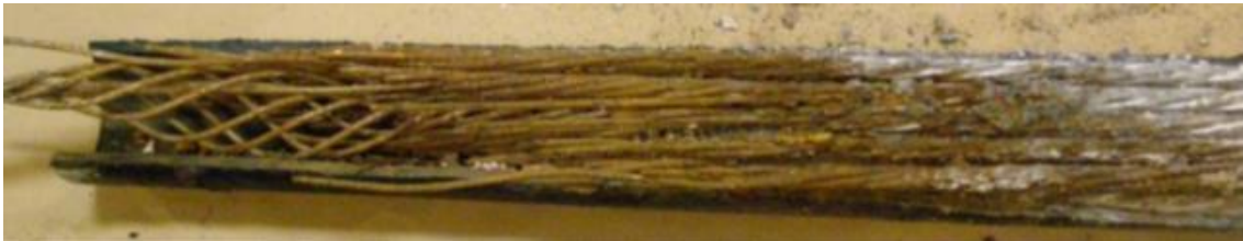
ID-20.2. Corroded tendon (Lau and Lasa, 2016).
