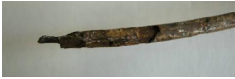
ID-18.1. Example of penetrating corrosion attacks observed on a wire of the failed cable (Bertolini and Carsana, 2011).
