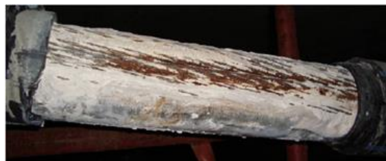
Figure 4.2.2.2. Example of whitish segregated grout embedding corroding strands in an Italian bridge (ID-18) (Bertolini and Carsana, 2011).
