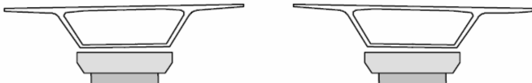
Figure 2.2.17. Sunshine Skyway Bridge (ID-11). Cross section of precast concrete sections for approach spans (Sayers, 2007).
