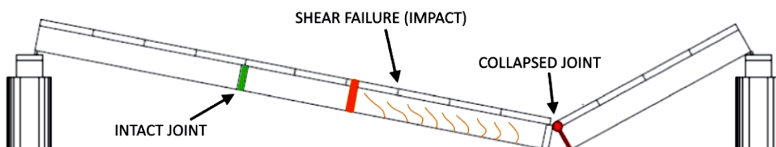
ID-5.3. Collapse mechanism (Bazzucchi et al, 2018).
