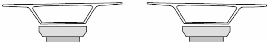
ID-11.3. Cross-section of pre-cast concrete sections for approach spans (Sayers, 2007).
