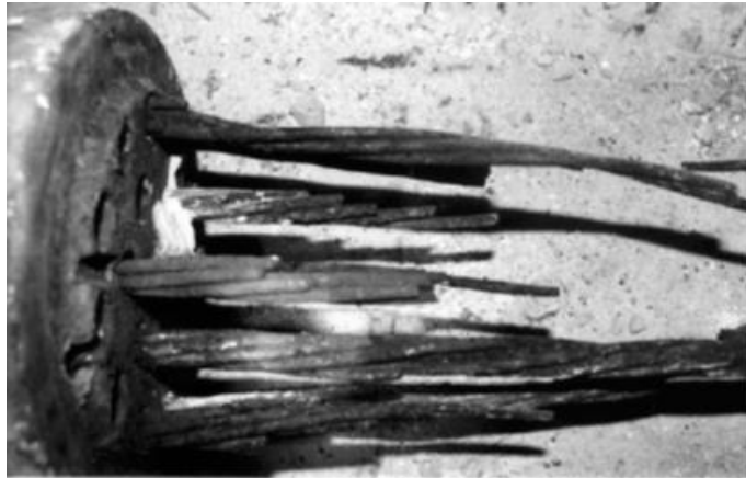
ID-17.1. Failed tendon of Niles Channel Bridge. June 1999 (Powers et al, 2002).
