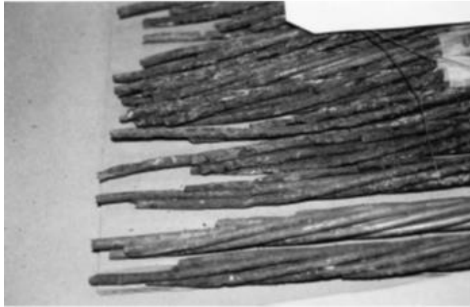
ID-9.3. Strand from one of the collapsed double-T's beams (Poston and West, 2005).
