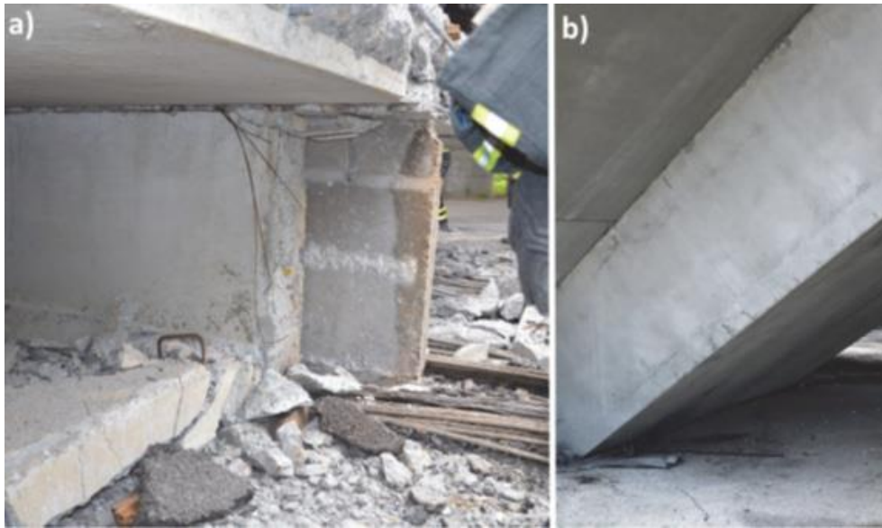
ID-5.4. Prestressing cables in the collapsed joint area (a); external concrete conditions (b) (Bazzucchi et al, 2018).
