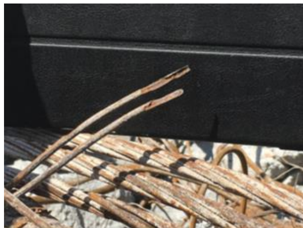
ID-6.8. Pit corrosion in the debris after failure (Nuti et al, 2020).
