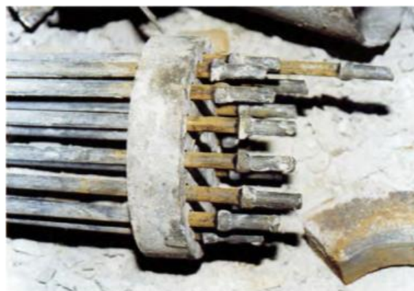
ID-30.3. Corrosion of wires at anchorage plate is greater than that exhibited inside ducts. (Dickson et al, 1993).
