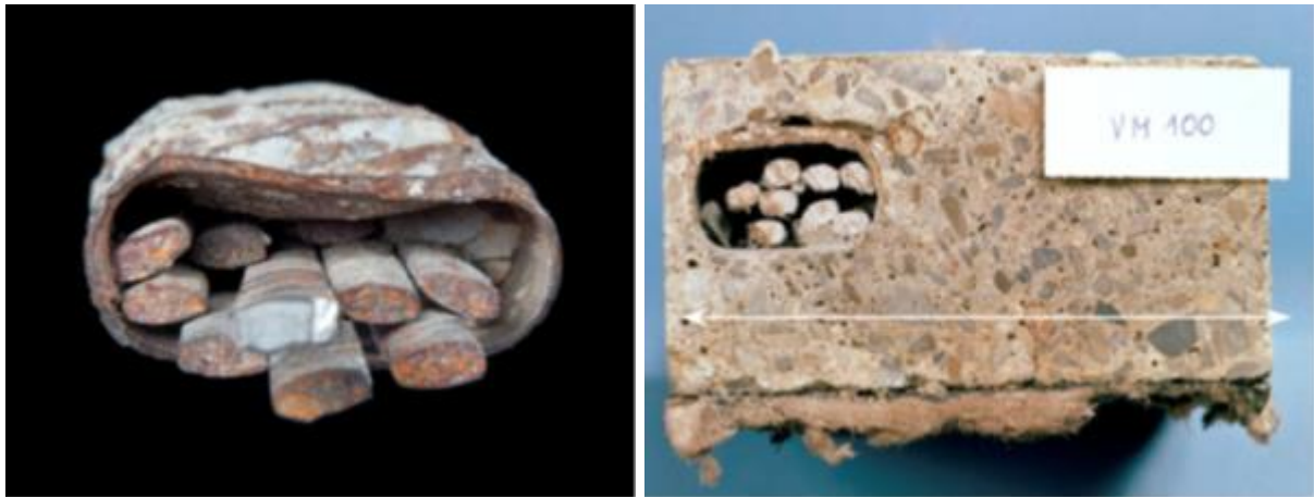
ID-19.7. Prestressing wires are almost not embedded in the protective grout (left) or insufficient grouted (right). Only one broken wire (left) shows a non-corroded brittle broken fracture surface. (Helmerich and Zunkel, 2014).
