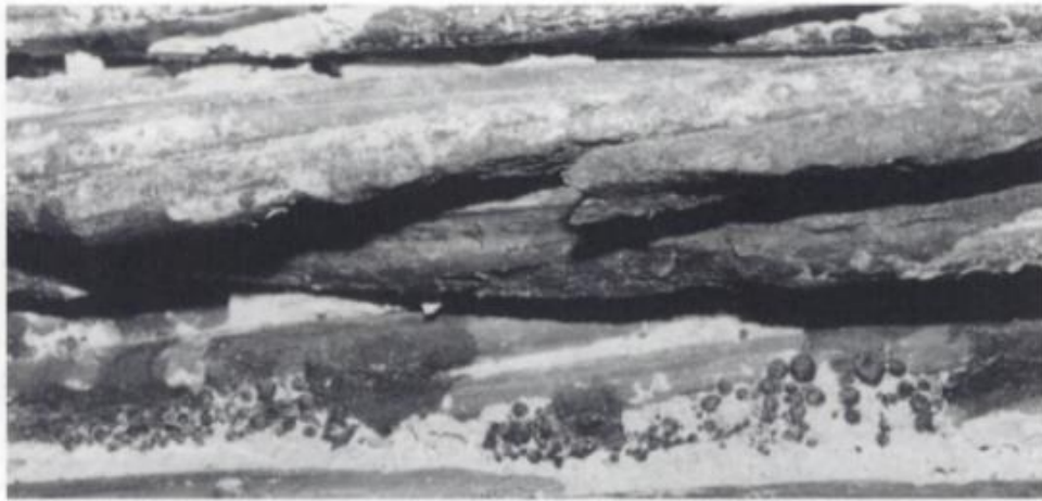
ID-7.4. Broken wire in one of the strands of Tendon 2 of Span 40-A (Venugopalan and Powers, 2003).
