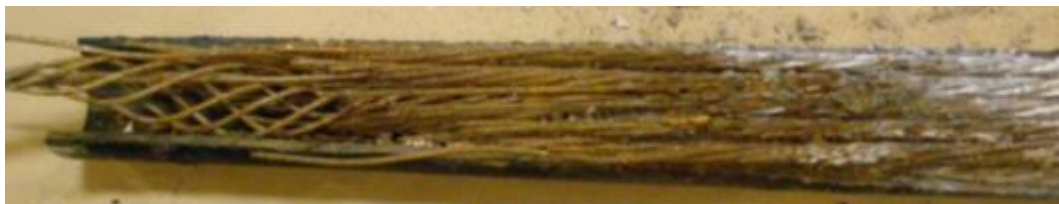
Figure 3.3.8. Corroded tendon in a Florida Bridge (ID-20) (Lau and Lasa, 2016).
