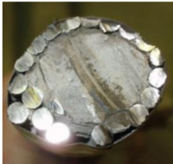
ID-3.3. Cross-sectional view of one of the most severely corroded tendons. Note the concave corrosion profiles at top and right. The central part is grout. The tape just visible around the outside as applied during recovery to keep the tendon together at the cross-sectional cut. There is no tendon duct (Papè and Melchers, 2011).
