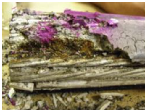
Figure 4.2.2.4. Corrosion of a strand embedded in deficient grout in Ringling Causeway Bridge (ID-15). Pink colour shows the pH indicator (phenolphthalein) sprayed on the grout surface (Lau and Lasa, 2016).
